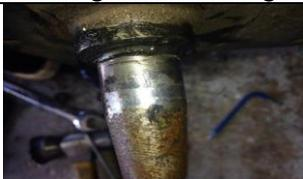
Last Veemag it was mentioned that stub axles on ball joint front ends have been found by Daniel Kleinig to be cracking. Here is another picture of a cracked ball joint stub axle. Again, please check your stub axles for cracks before the next race meeting. This could be another scrutineering item at the next race meeting (Col, Chris?).
